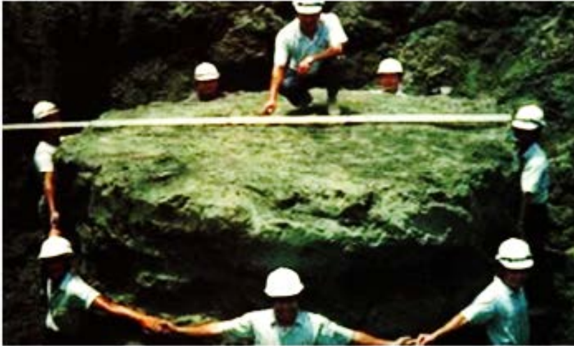
Figure 2.6. The column formed using Jet-3 [7].
