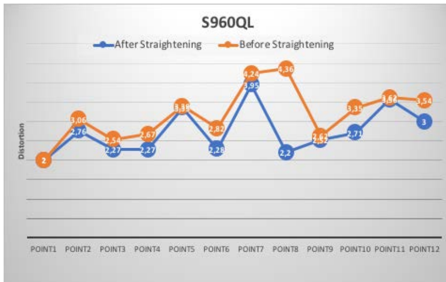
Figure.4. (b). Distortion measurement in (mm) before and after straitening for S960QL,
