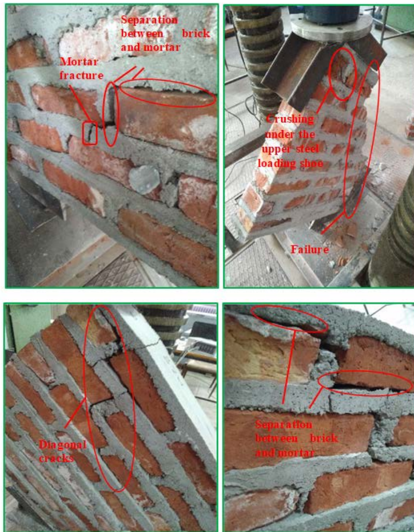
Figure 7. Cracks and failure modes in the MWRM samples
