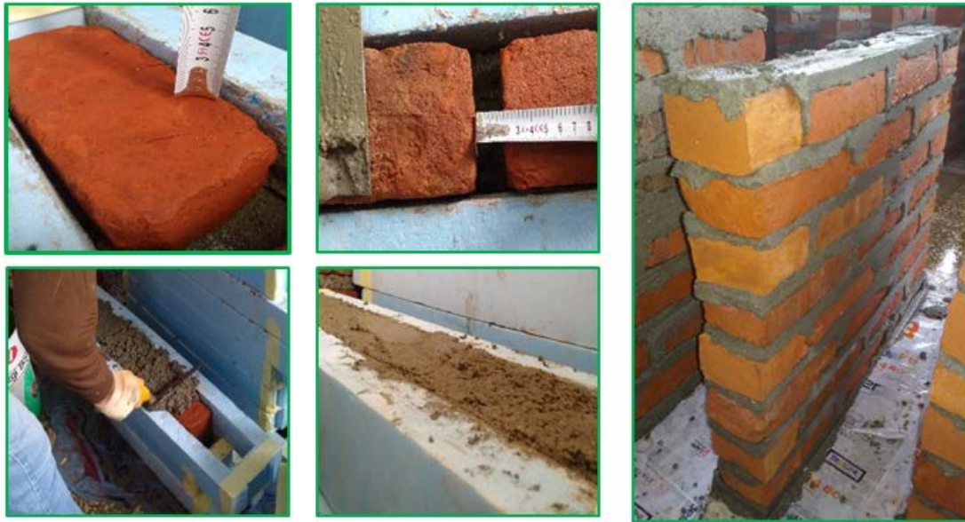
Figure 5. Preparing of masonry wall samples
