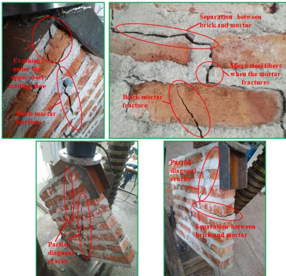
Figure 9. Cracks and failure modes in the MWFM2 samples
