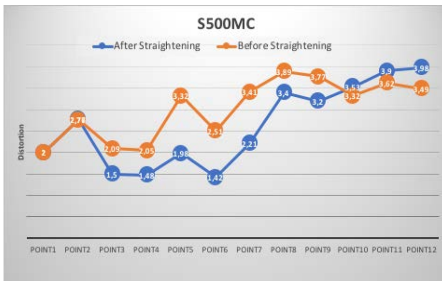
Figure.4. (b). Distortion measurement in (mm) before and after straitening for S500MC,
