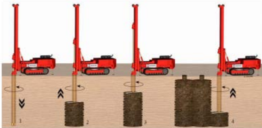
Figure 2.3. Schematic representation of the Jet Grouting System [7].
