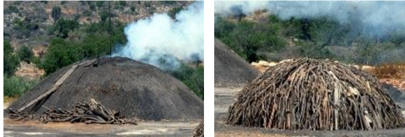
Figure 1. An active charcoal kilns made of piled up timber (left) and the piled up timber before covered by iron sheets and sand
